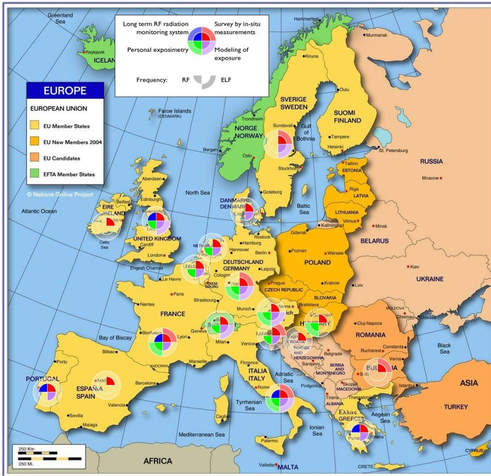
**Fig.1.** EMF public exposure assessments in the European countries. The size of circles represents the level of activity on the corresponding exposure methods as: i) long term RF radiation monitoring systems, ii) survey by in-situ measurements, iii) personal exposimetry and iv) exposure modeling to RF and/or ELF range.
