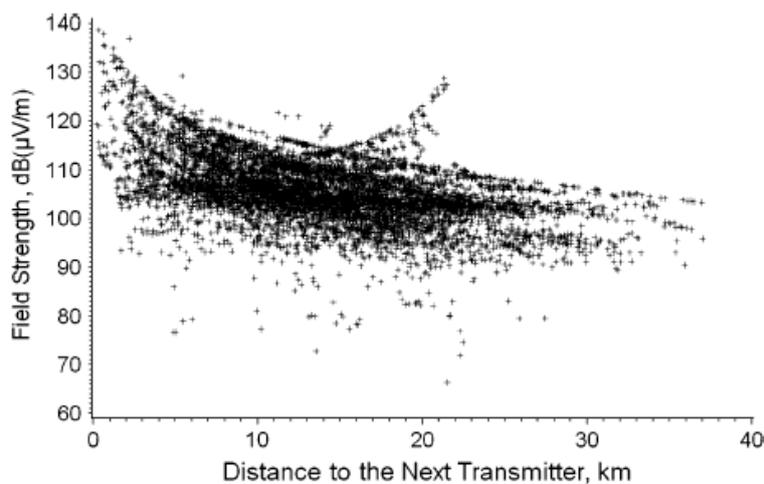
**Fig.2.** Scatter plot of total radio frequency electromagnetic fields in relation to distance of study subjects' place of residence to the nearest main transmitter, Germany, 1984–2003. For example, 120 dB(μV/m) = 1 V/m. (from Merzenich, 2008)
